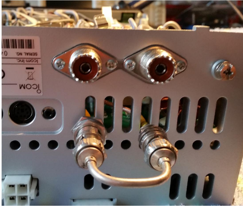
Figure 3: RX out - RX in with the BNC jumper cable
